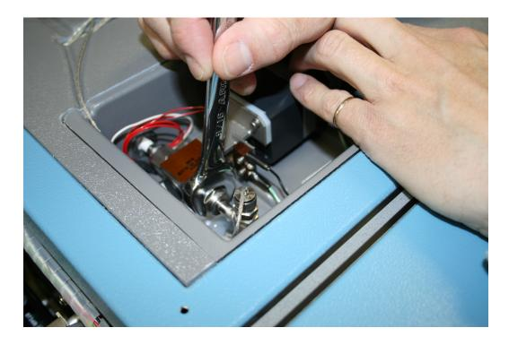
6. When loosening the front nut, be careful not to hit the switch mounting bracket.
