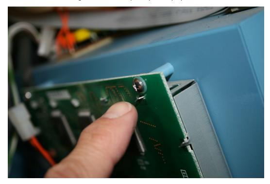
14. Now using a number 1 Philips head screwdriver with a 90° bend or a ratchet drive, loosen but do not remove the top left-hand and right-hand screws.
