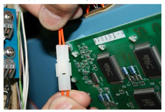
8. Pull the cable connectors apart, you may need to use a small flat head screwdriver to help.
