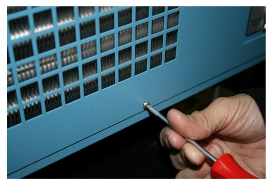
3. Remove the reservoir fill port cap.
