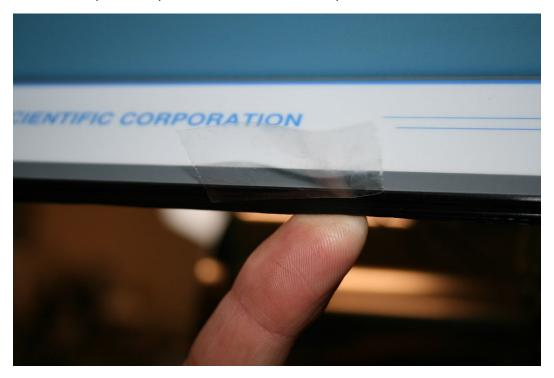
24. Get the new liquid crystal display assembly and remove the clear film protective cover.
