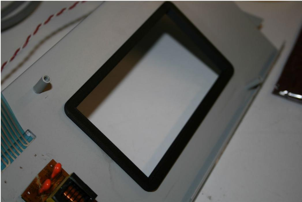
23. Remove the protective film from the new LCD board module.
