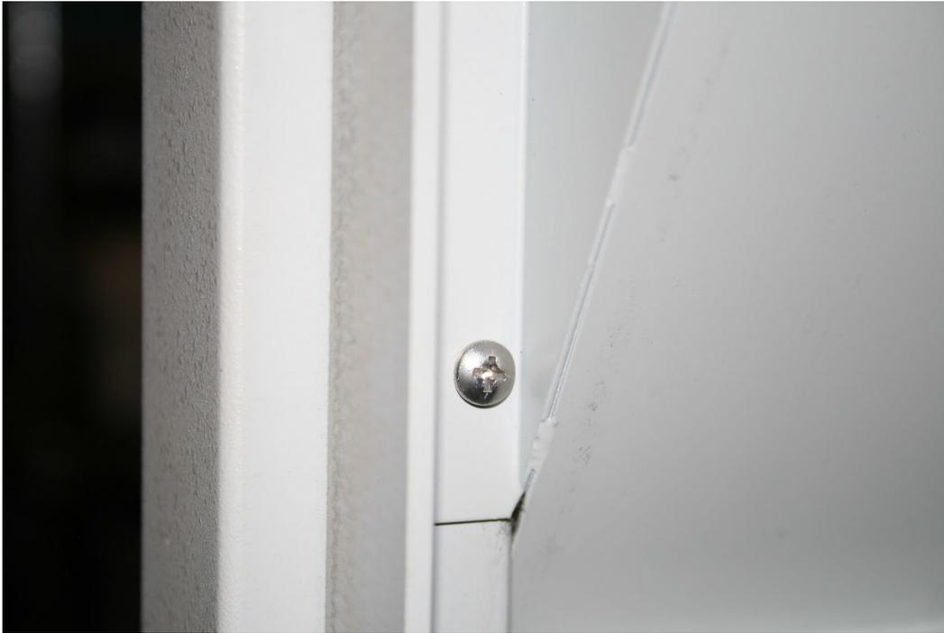
15. Use the #2 Phillips head screwdriver and remove all four screws and save them for later installation.
