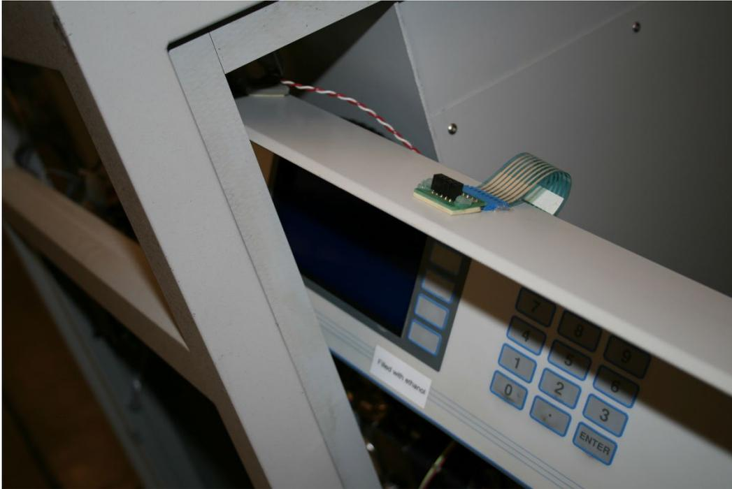
29. While holding the control panel hood assembly in place insert the four Phillips head screws that were saved from earlier in this procedure.
