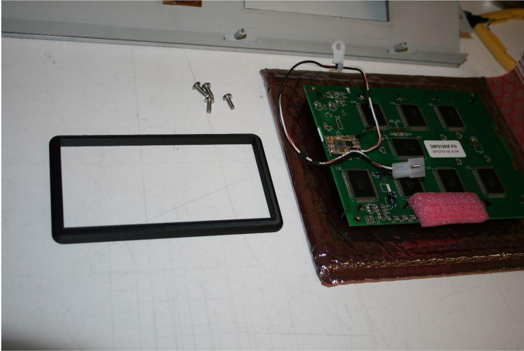
21. Takt the bezel and make sure that the small side goes towards the rear side of the control panel hood assembly.
