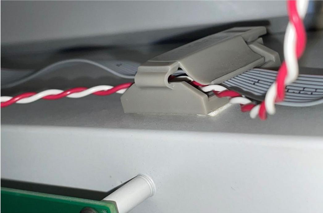
9. Pull it open and remove the red and white wire and the ribbon cable.
