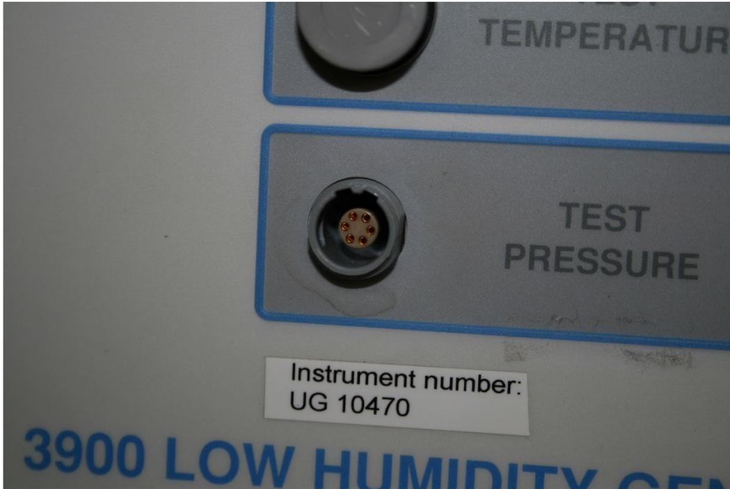
43. Screw on the connector cover so that it flips upward as well. Using the same two wrenches as before tighten the nut at the rear of the connector.
