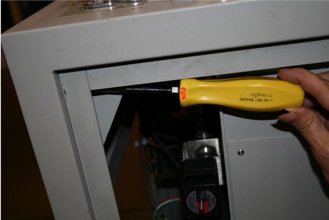
31. Then insert the screws, top and bottom on the left side.
