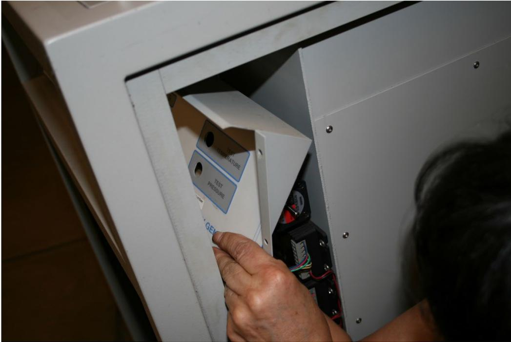
17. Using the wire cutters, cut all four wires on the inverter board assembly.
