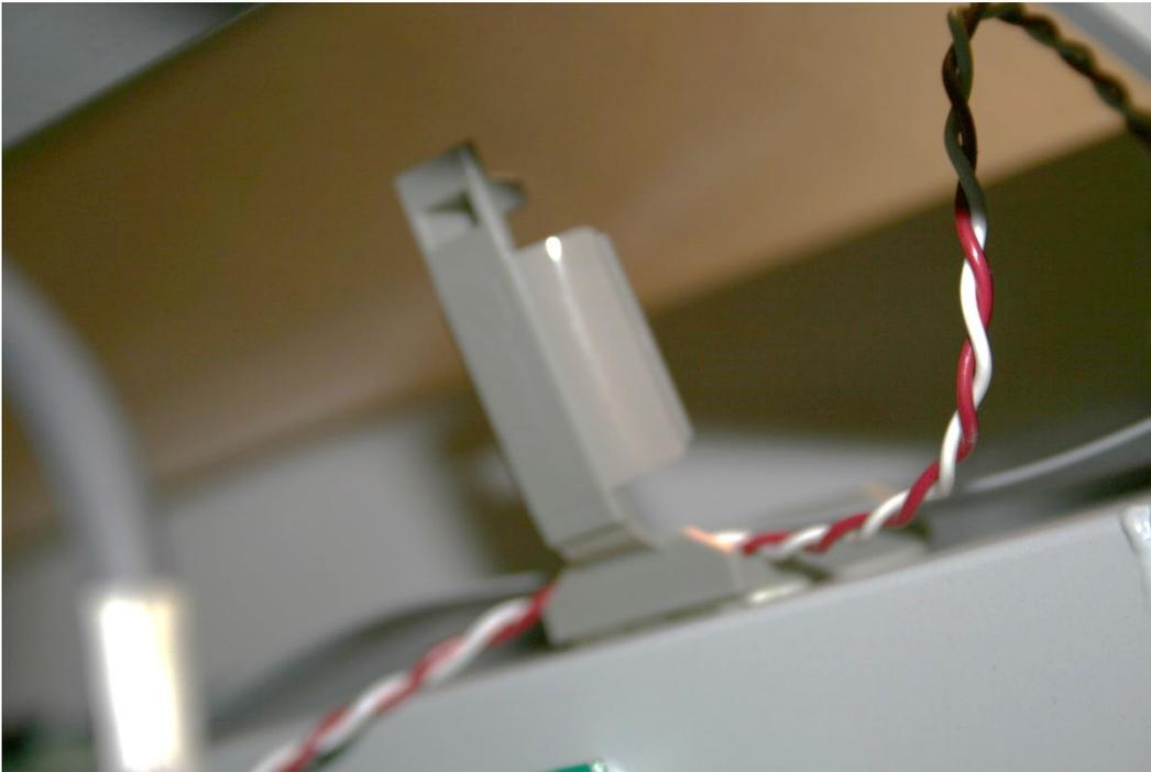
10. Disconnect the red and white wire using the small flat head screwdriver.
