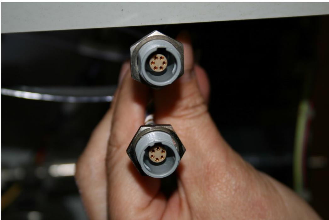
38. Push through the Test Temp single slot connector at the top.
